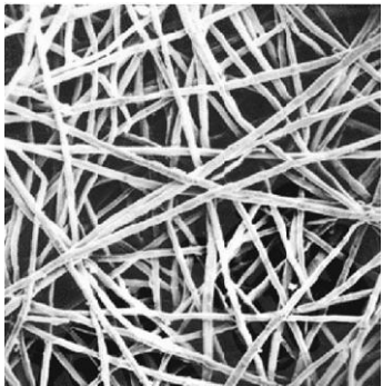
图 3 不锈钢纤维烧结毡 Fig. 3 Sintered felt of stainless steel fiber
