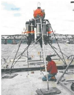
图 5 1996 年拟用于旧金山的 USGS GEOPROBE 三脚架 Fig.5 USGS GEOPROBE tripod being readied prior to deployment in San Francisco Bay, CA in 1996
